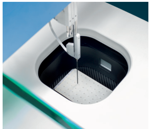
Access of pipetting tips to the shaking microtiter plate in the BioLector®
